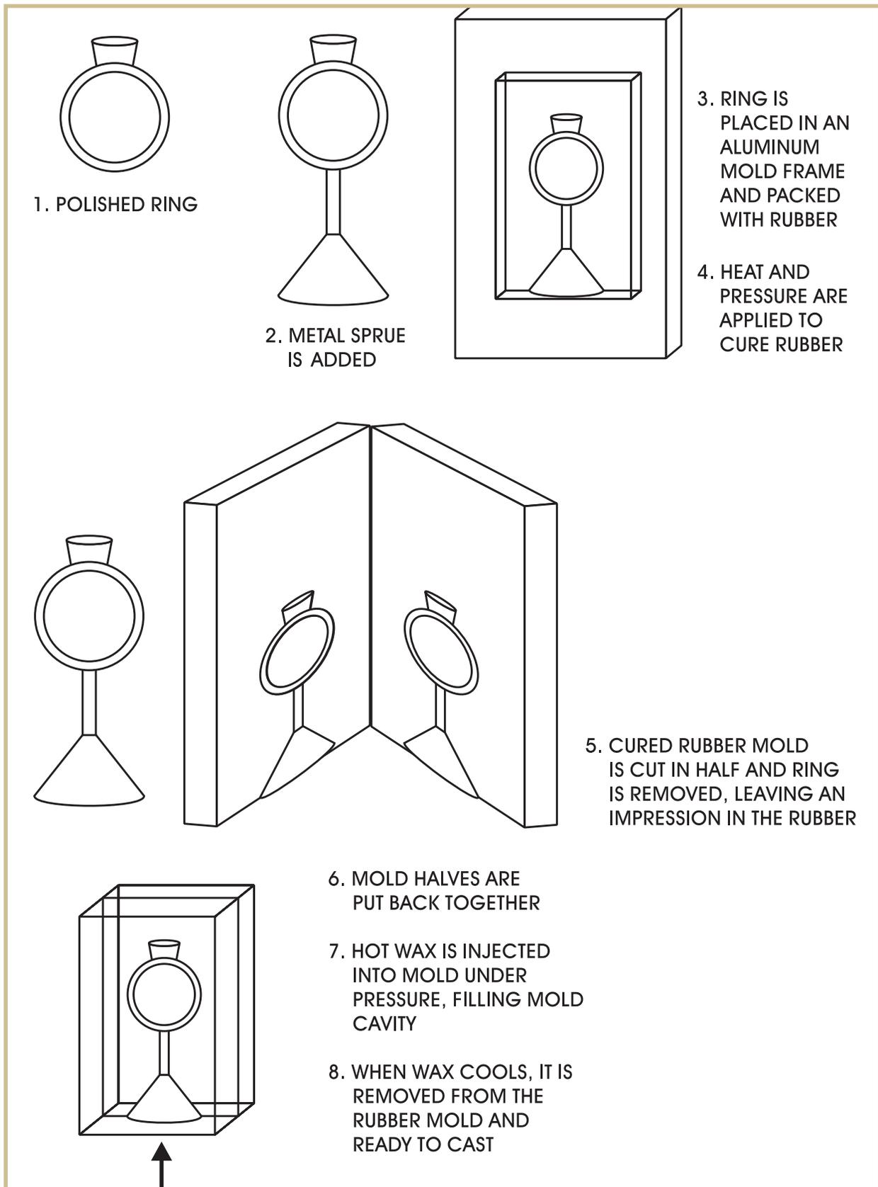
FIGURE 1—An Overview of the Moldig Process
