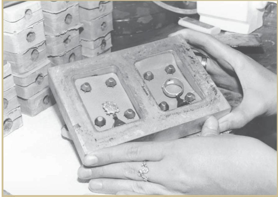
The pressure you place the mold under won't be enough to force the precut rubber into any stray holes in the object. It's therefore important to pack any holes with small pieces of mold rubber. In Figure 5, the object in the left mold is flat, and can simply be covered with another piece of rubber. The object in the right mold, however, requires additional pieces of rubber packed into the center of the ring and any cuts or crevices.
