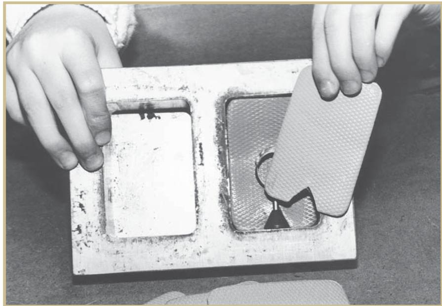
After you cut these areas away for the sprue base, place the third and fourth pieces into the frame. You're now ready to lay the jewelry item in to be molded. The areas you've cut away to accept the sprue will help to hold the item in place.
