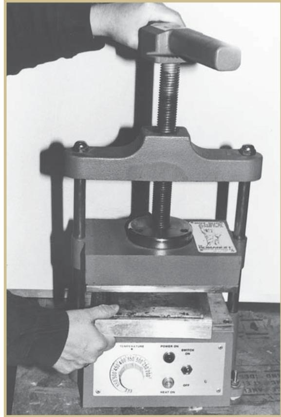
*FIGURE 8—Removing Mold with Tongs*
