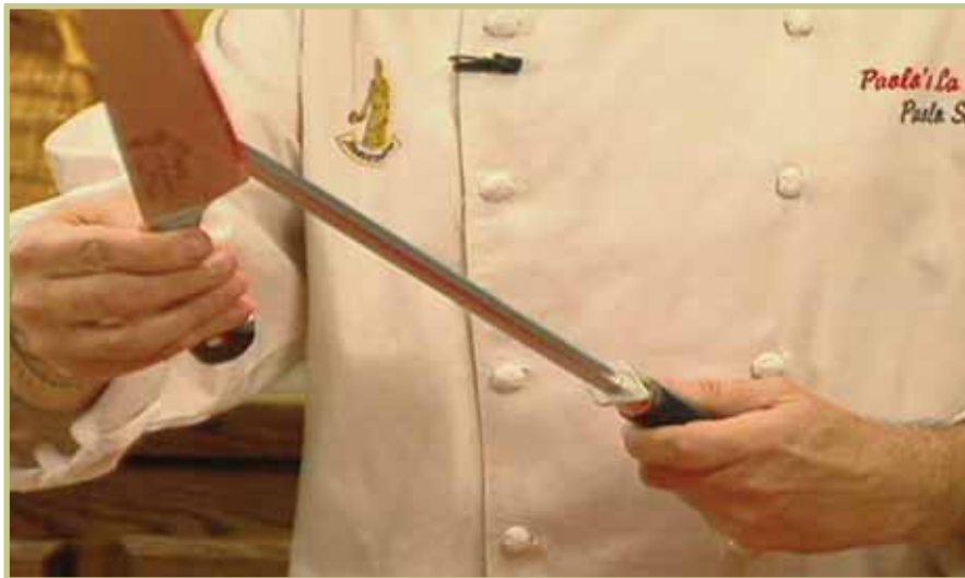
FIGURE 17 —One method of honing a knife involves holding the steel at this angle.
