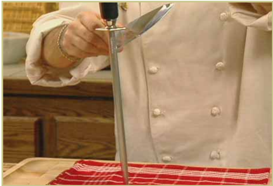
FIGURE 19 —For a more stable method of honing, place the tip of the steel against the counter.
